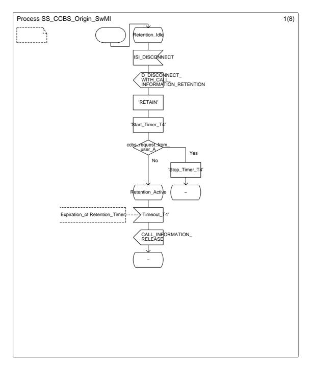
Figure A.1: Originating SwMI process (sheet 1 of 8)
