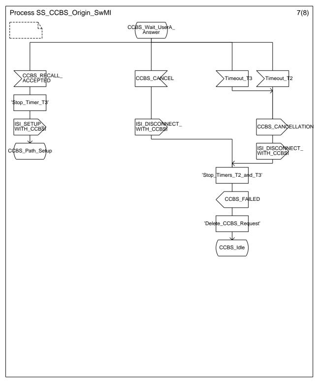
Figure A.1: Originating SwMI process (sheet 7 of 8)
